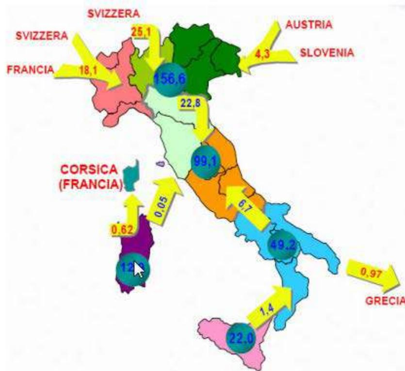
Fig. 3: external and internal energy exchange (arrows) and consumption (circles) for Northern, Central, Southern, Sicily and Sardinia zones in Italy in 2007 (figures are in GWh).
